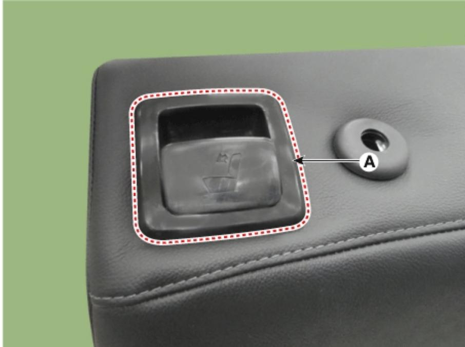
5. Remove the rear center seat belt cover (A) by using a remover.
