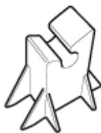
10. Pull out and remove the rear seat headrest guides (A) while holding both sides of the lower part of the guides.
