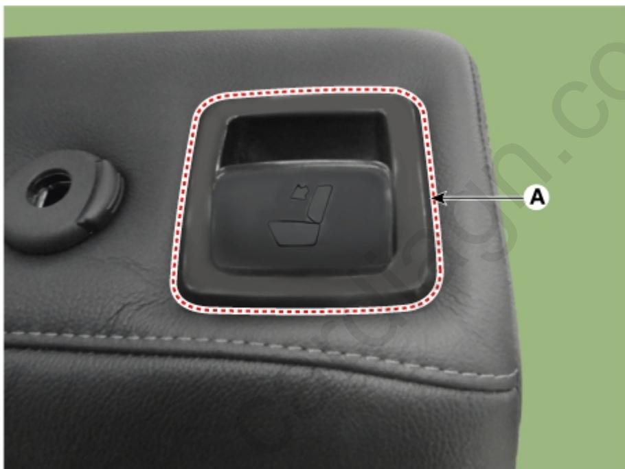
5. Remove the child anchor cover (A) by using a remover.
