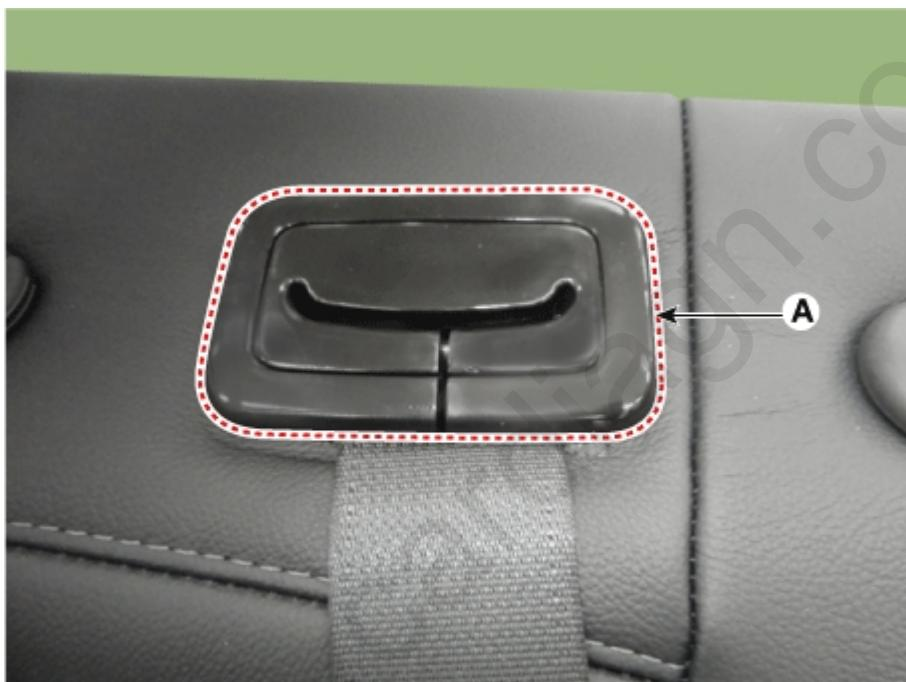
6. Remove the child anchor cover (A) by using a remover.
