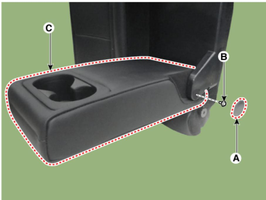
9. Remove the rear seat armrest back board (A).
