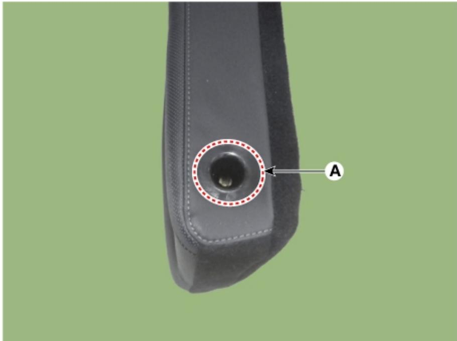
4. Remove the rear seat back folding knob cover (A) by using a remover.
